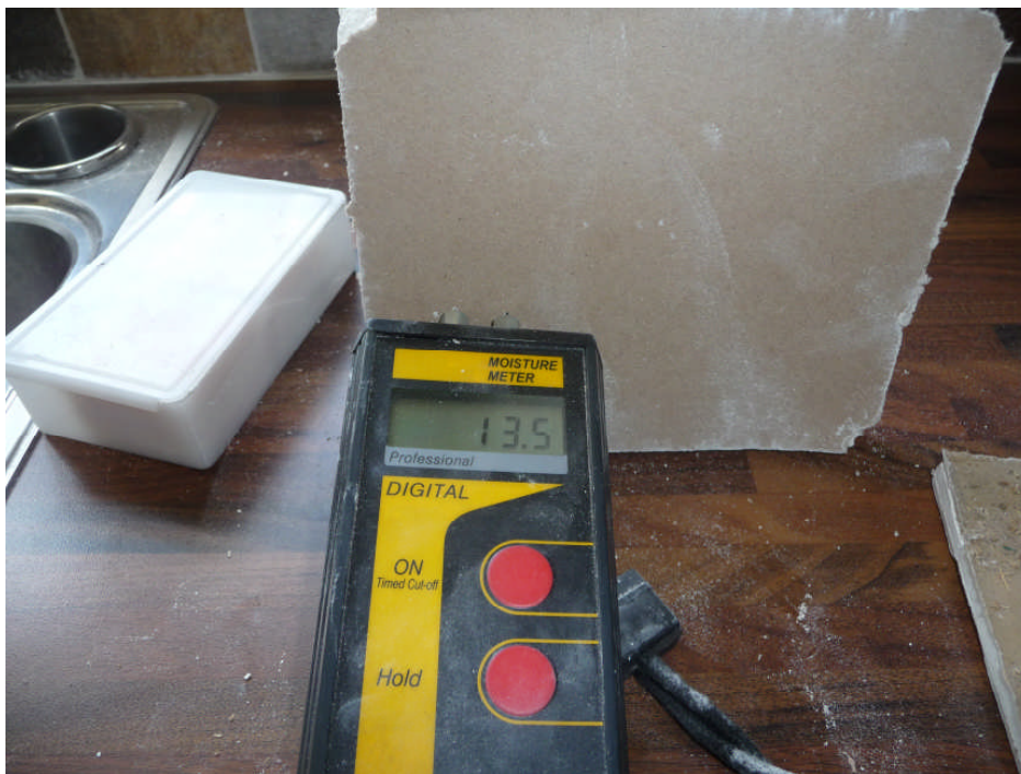
Photo 4 Bottom layer plasterboard showing moisture content
