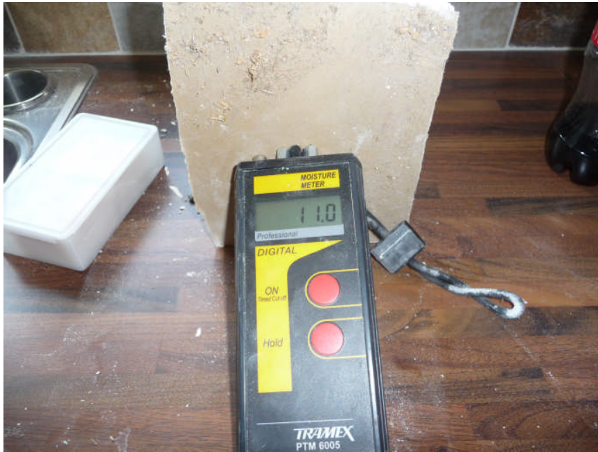
Photo 4 Bottom layer plasterboard showing moisture content
